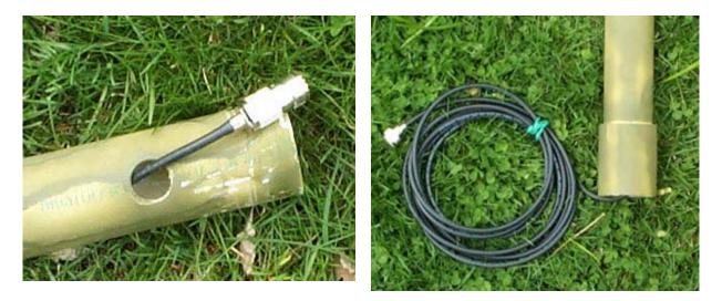
Install pipe coupling to one end of the pipe as seen above. Install a coupling to the remaining pipe as well. The couplings need not be glued... in fact I didn't glue any of the caps or couplings and they seem plenty sturdy for the purposes of the support mast.
