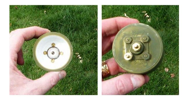
Cut off the head of a 1" #6 brass screw and solder it in the center post of SO-239.
